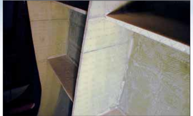
Sailing catamaran interior structural bulkheads shown using Structiso cored sandwich construction.
