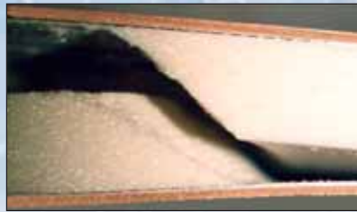
Typical shear failure shown within foam cored sandwich panel.
