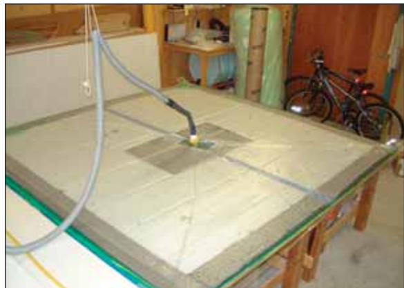
A Nida-Core installation, using vacuum bagging, is shown. Note the alternative core used as a perimeter enclosure for edging purposes. This method retains the sound-damping qualities of the part.
